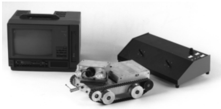
Figure 7-4. Tools of the trade. Featured is a robotic duct inspection and cleaning system with remote control. Inspects, cleans and records the job. Courtesy: Indoor Environmental Solutions.
