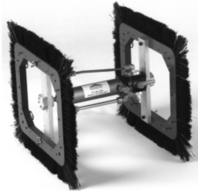
Figure 7-3. Tools of the trade. Featured is a “duct walker,” a brush system that fits snugly into sheet metal, insulated or ductboard ducts and automatically brushes all sides and corners. Courtesy: Indoor Environmental Solutions.
