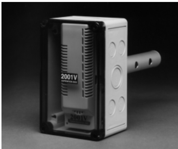
Figure 4-11. A carbon dioxide sensor. When carbon dioxide builds to a trigger point, the ventilations system provides more outside air to the space, a process called demand control. Courtesy: Telsaire Systems, Inc.
