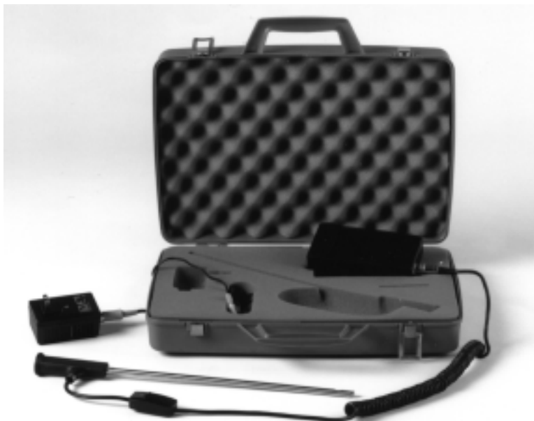
Figure 7-10. A boroscope used for “before and after” records—ductwork inspection and to demonstrate the work has been done satisfactorily. Courtesy: Indoor Environmental Solutions.
